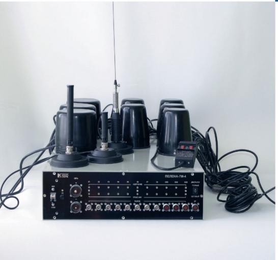
The jammer is used to interfere with radio-controlled explosive devices (RCED) and as a protection against unauthorized phone-tapping by means of special radio sets. It is used to jam high-power signals covering a wide frequency band of the most commonly used commercial devices (warning systems, radio stations, etc.) to Wi-Fi wireless data transmission systems; it is also used to enhance the protective efficiency within the cellular bands.
