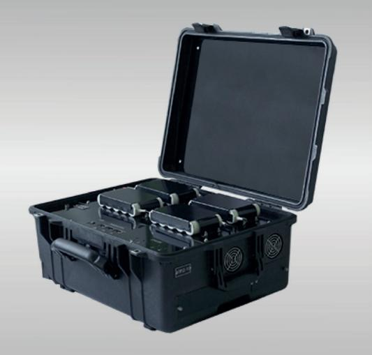
The jammer can be effectively used as a portable protective device: it can also be used to protect vehicle passengers. The jammer is used to interfere with radio-controlled explosive devices (RCED) and as a protection against unauthorized phone-tapping by means of special radio sets. It is used to jam signals in the required frequency band, and when additional protection of the jammer against external mechanical damage is required.
