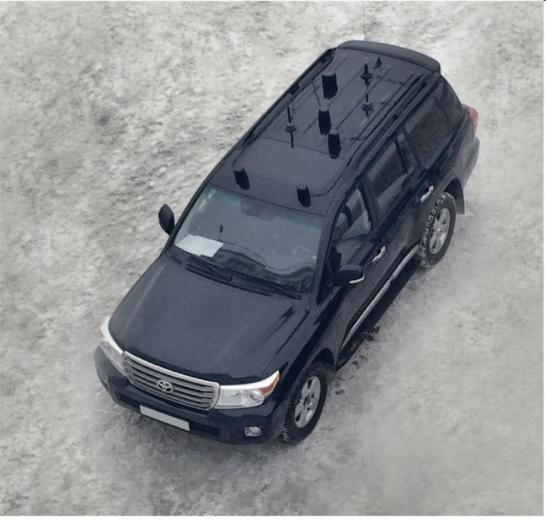
The jammer is used as passengers' protection against phone-tapping by means of special radio sets. It is also used to interfere with operation of the radio-controlled explosive devices (RCED). It is used to suppress high-power signals in the extended frequency band, and also to enhance the protective efficiency within the cellular bands.
