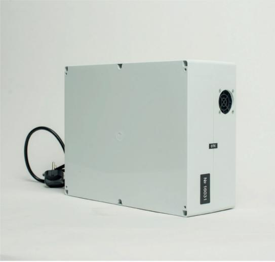
The jammer is designed to counteract cellular communication of GSM 900/1800, 3G, 4G-700, 4G/LTE, WiFi and Hi-WiFi standards in the individual limited areas.
