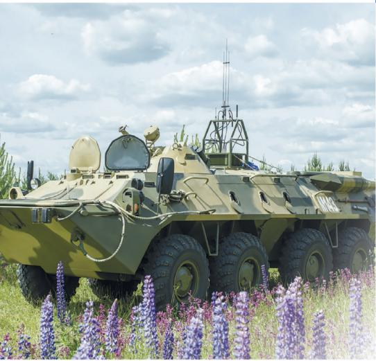
The jammer serves to interfere with radio-controlled explosive devices (RCED) by means of a signal within the whole operating band: it is mounted on the vehicle and serves to protect from RCED when moving and in the stationary position. There is a structure to attach a bullet-proof vest to protect the equipment against any mechanical damage, which makes it possible to effectively use the jammer during warfighting.
