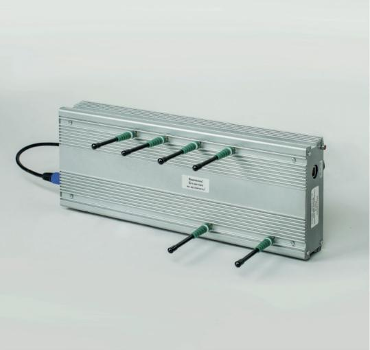
SHTIL-KOM integrated solution for jamming and detecting cell phones is used to support the set mode of information security of the focused objects by jamming cellular communication channels with the allowed list of subscriber devices of cellular carrier networks still operating in the allowed bands.
